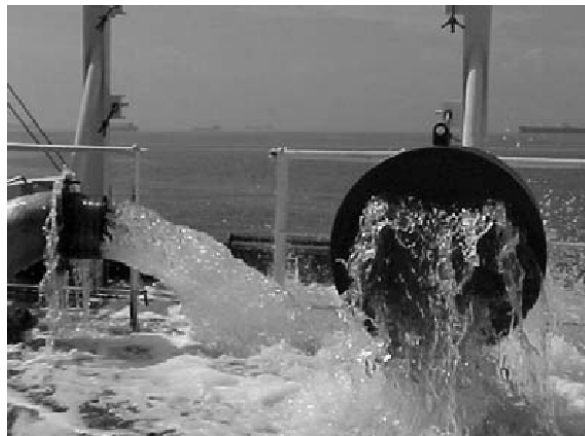
Figure 6. Example of an adverse overflow situation
