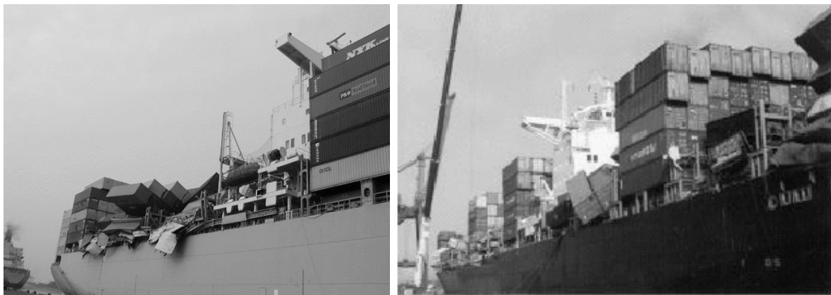
Fig. 1: Representative Container Damages
