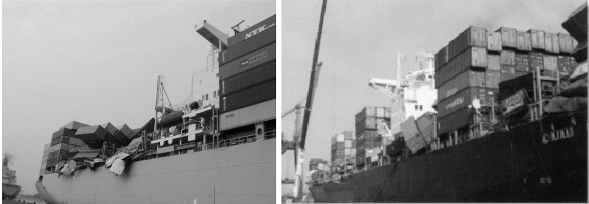
*Figure 14: Representative Container Damages*
